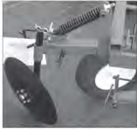
Spring loaded covering disks
